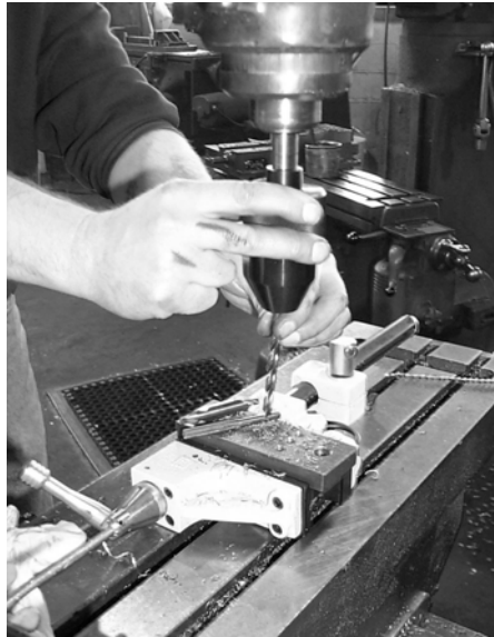
2. Insert new drill. Push tapered part up. Drill is locked in place.
